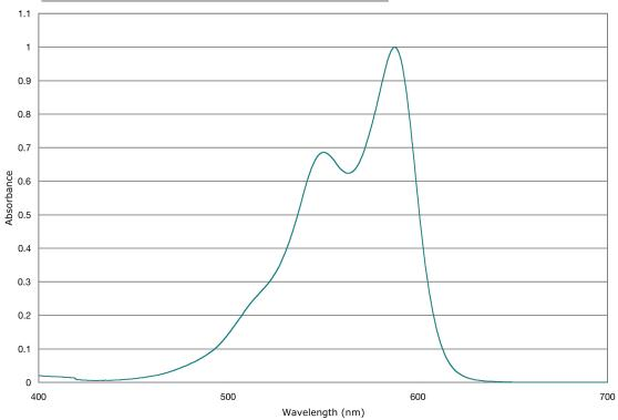
VIS588C is one of many Visible Dyes for solvent systems available through QCR Solutions Corp. We offer NIR dyes in a wide spectral range between 400nm - 700nm for various applications. Our large library of absorbers contains narrow notch to broad band absorption curves. These NIR dyes can be used singly or in combination to create custom spectral filters.
